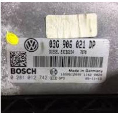
Figure VW PASSAT B6 ECU ENGINE CONTROL UNIT BKC ENGINE 03G906021 DP 1.9TDI 2006
